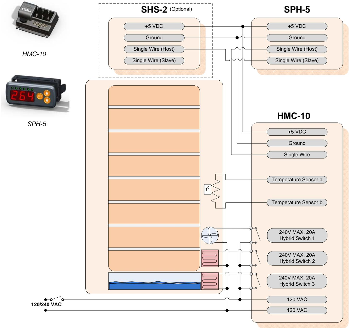
The **HMC-10** has 3 Hybrid switches capable of switching up to 240 VAC at 20 amps. The built in transformer allows the **HMC-10** to be directly connected to the mains. It's internal regulators provide 5VDC out to power peripherals controllers. It offers Renau's single wire communication protocol to reduce the cost and complexity of the wire harness.
